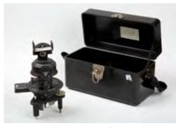
Astrocompass used by the navigators of British bomber planes
